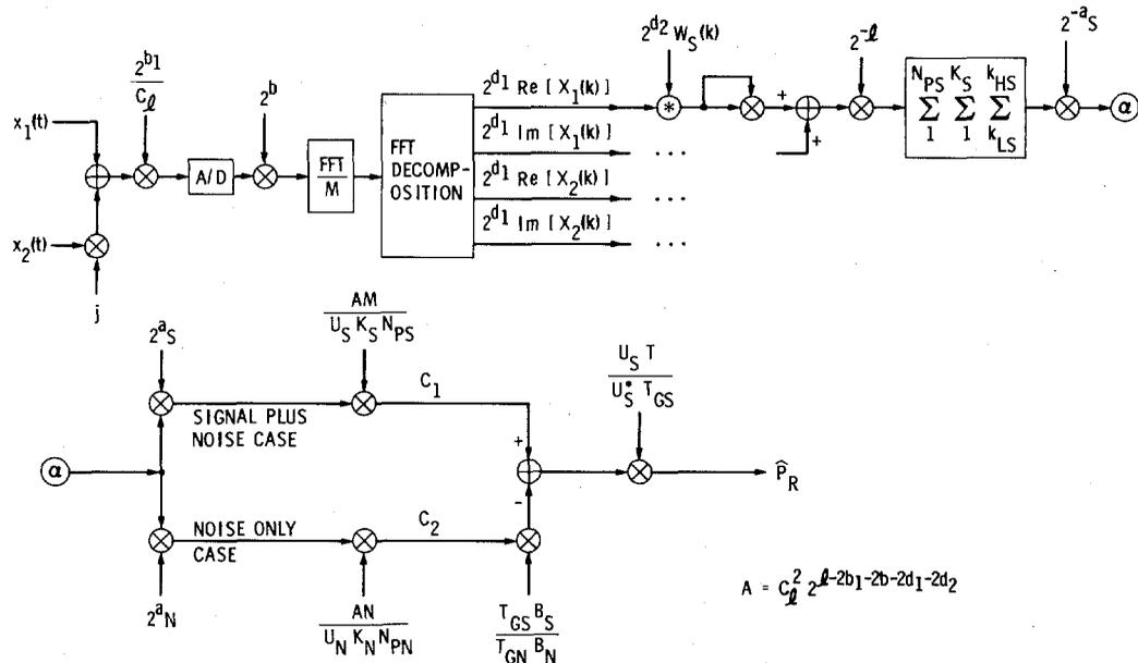
Fig. 2. A realization of the DSP using Welch's power spectrum estimation.
