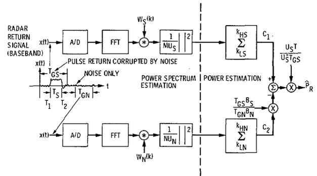
Fig. 1. Signal processing system for a digital signal power processor (DSPP) using Welch's power spectrum estimation.
