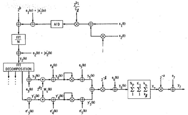
Fig. 3. Roundoff error sources in the DSPP shown in Fig. 2. In the triple summation,  $N_p = N_{pS}$ ,  $K_1 = K_S$ ,  $k_h = k_{HS}$ , and  $k_l = k_{LS}$  for the signal-plus-noise case;  $N_p = N_{pN}$ ,  $K_1 = K_N$ ,  $k_h = k_{HN}$ , and  $k_l = k_{LN}$  for the noise-only case.
